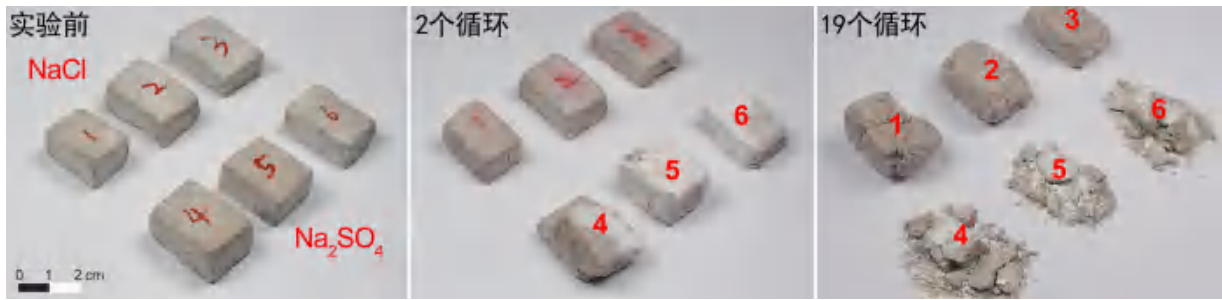
图9 NaCl (1-3)和 Na 2 SO 4 (4-6)循环过程中岩石样品的外观变化 Fig. 9 Appearance of rock samples during NaCl (1-3) and Na 2 SO 4 (4-6) salt aging test
